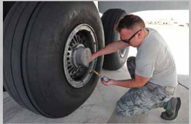
Master Sgt. George LaCome, 151st Maintenance Group crew chief, checks the tire pressure on a KC-135R during a preflight inspection at Andersen Air Force Base, Guam, prior to the six-person crews aeromedical-evacuation mission in the Pacific theater from Feb. 8-25, 2017.
